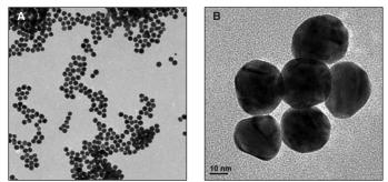
Figure 1: TEM images of gold nanoparticles. A) 15nm spheres, at 40000X B) Close up of 30nm spheres showing the monodispersity.
