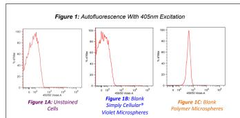
**Figure 1A, 1B, 1C:** With 405nm excitation, unlabeled Simply Cellular® for Violet Laser beads demonstrate autofluorescence resembling that of unstained cells. Unlabeled polymer beads demonstrate greater autofluorescence with violet excitation.
