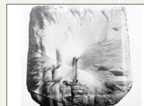
An x-ray topograph of a man made high-temperature/high-pressure diamond single crystal. Image courtesy of The Electrochemical Society, Inc.
