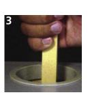
Insert dip stick in tank for 10 seconds.
